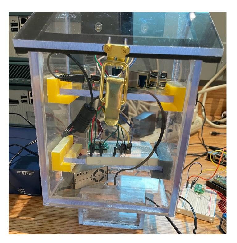
Figure 7 – Prototype of Enclosure with Modular Design for Additional Sensors
