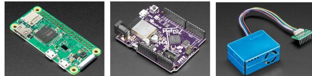
Figure 3 – Sensors Utilize Commonly Available Microcontrollers and Microprocessor Boards and Sensor is a Plantower PMS Sensor
